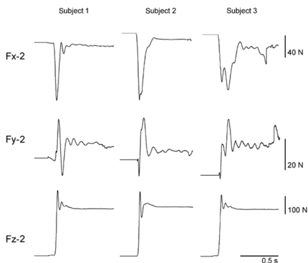
Figure 3. Averaged traces of moments recorded from force plate-2. Traces for three subjects are presented as in Fig. 2. There was a difference in the waveform of anteroposterior (Fx-2) and lateral (Fy-2) direction moments among the subjects, while vertical (Fz-2) moment also showed relatively constant waveforms with two major upward peaks
