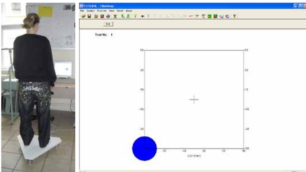
Figure 1. Task execution: hit the target by shifting COM in one of the four directions according to position of stimulus on the screen while standing on unstable spring-supported platform equipped with PC system for feedback monitoring of COM movement ([www.fitronic.sk](http://www.fitronic.sk))
