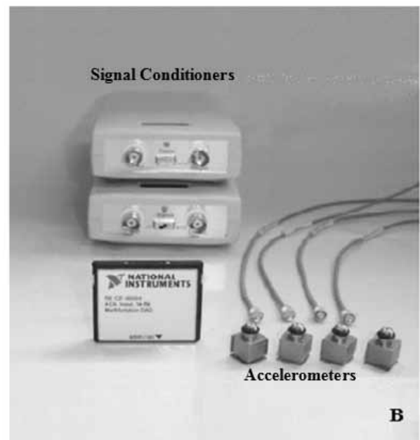
Figure 1. (A) Accelerometer Brüel & Kjær, model DeltaTron ® 4507 B 005. All dimensions are in millimeters. The “arrow” shows to the direction of acceleration (image taken from the manual of the accelerometer), (B) Set of four accelerometers Brüel & Kjær, model DeltaTron ® 4507 B 005 and the signal conditioner
