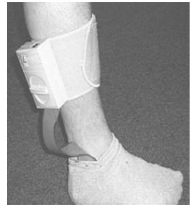
Figure 2. Pressure sensor inserted into sock
