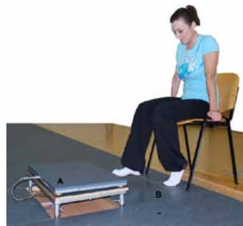
Figure 2. The experimental setup. Rhythm reproduction with the lower limb on a Kistler force plate (B)
